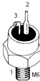
1 = Anode, 2 = Cathode, 3 = Gate
